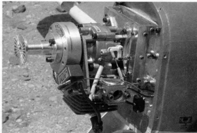
Fuji engine in John Sands' plane has a plywood engine mount reinforced with aluminum angle stock (above right). Wiring is for a servo actuated kill switch.
