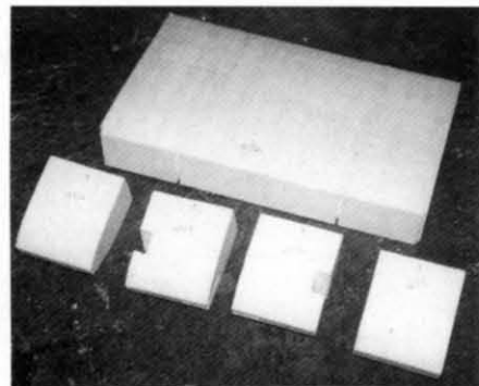
These are the foam core parts for the wing center section. The outer wing panel cores will complete the wing. The tail surfaces are foam cores as well. Ply pieces for brace and landing gear are added later.
