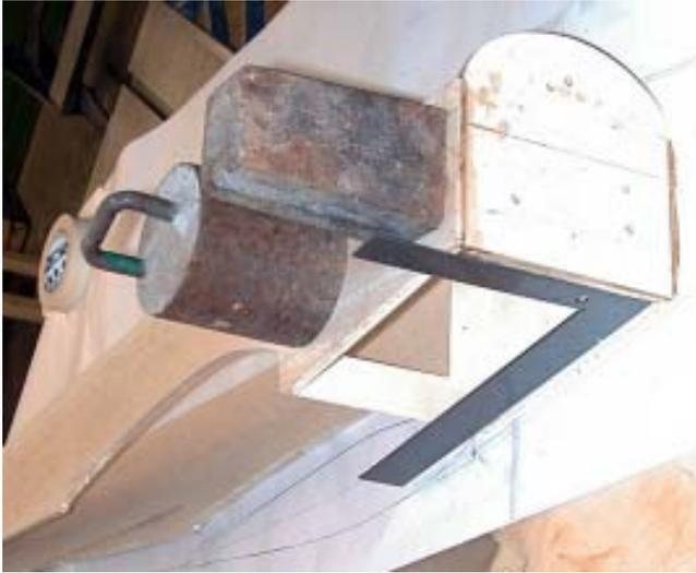
of doubler even with wing cutout on fuse sides. Glue wing saddle doubler in place behind F2, making sure that it doesn't go past F4's front edge.
