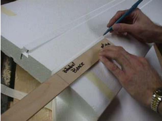
❑ Draw a vertical line at the center of the dihedral brace. Test fit the dihedral brace into both wing halves, making sure that the flat side goes towards the top of the wing. It should fit against the two spars when the center line is even with the end of the wing. sand carefully if needed.
