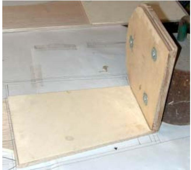
bottom on other side. This allows former to be sanded flush with fuse bottom prior to installing fuse bottom sheeting.
