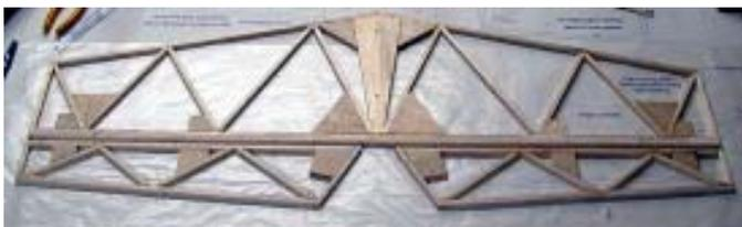
❑ When glue has dried, remove Stab from plans, and sand top and bottom even.
