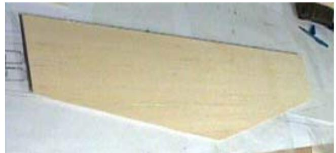
❑ Glue 3/8" tri stock to LE of both Elevators. Be sure tri stock is centered on elevators.
