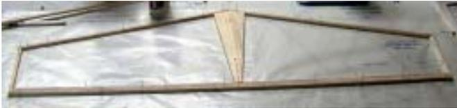
❑ Pin 1/4" precut stab center section over plans. Leave point on front of Stab. This will be sanded flat for exact fit when stab is fitted to Fuse.
