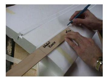
Draw a vertical line at the center of the dihedral brace. Test fit the dihedral brace into both wing halves, making sure that the flat side goes towards the top of the wing. It sould fit against the two spars when the center line is even with the end of the wing. sand carefully if needed.
