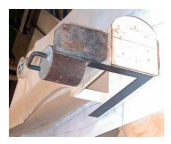
of doubler even with wing cutout on fuse sides. Glue wing saddle doubler in place behind F2, making sure that it doesn't go past F4's front edge.
