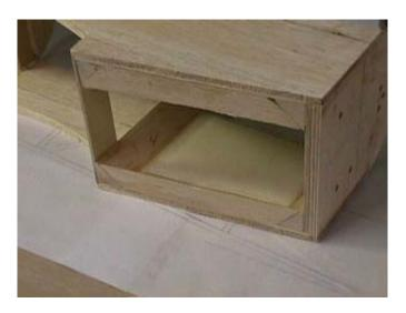
☐ Sand bottom of front fuse section and epoxy 1/4" ply FFB in place. Be sure landing gear holes are towards
