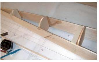
It will be much harder to do with bottom of fuse and top stringers in place. If you use hardwood rails as shown on the plans, you can cut a notch in the op of the fuse sides to mount the rails in to, then reinforce with tri stock.
