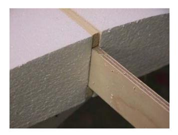
□ Epoxy in 1/2" x 1/4" x 34" spruce spars in slots in wings, one top and one bottom. Be sure the spars are flush with the surface of the wing and don't protrude so that they do not interfere with sheeting when it is applied. You may want to wrap wax paper around the dihedral brace and have it in place while the spars dry to ensure a tight fit.
