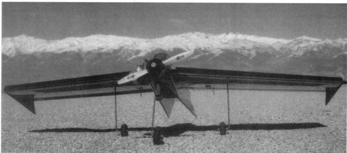
And obvious requirement of tails on the bottom side of a plane is the need for stalky landing gear—but you can swing a huge prop!
