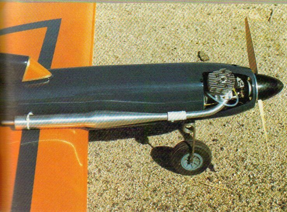
ABOVE: Two Desperado 3000's flight line ready. LEFT: S.T. 3000 shown with Mac's header and pipe, proved to be an excellent combination.
