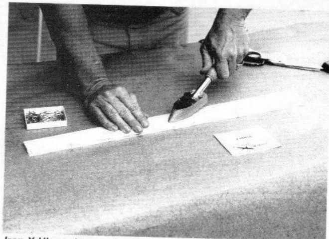
Iron X-Hinge down onto elevon.
