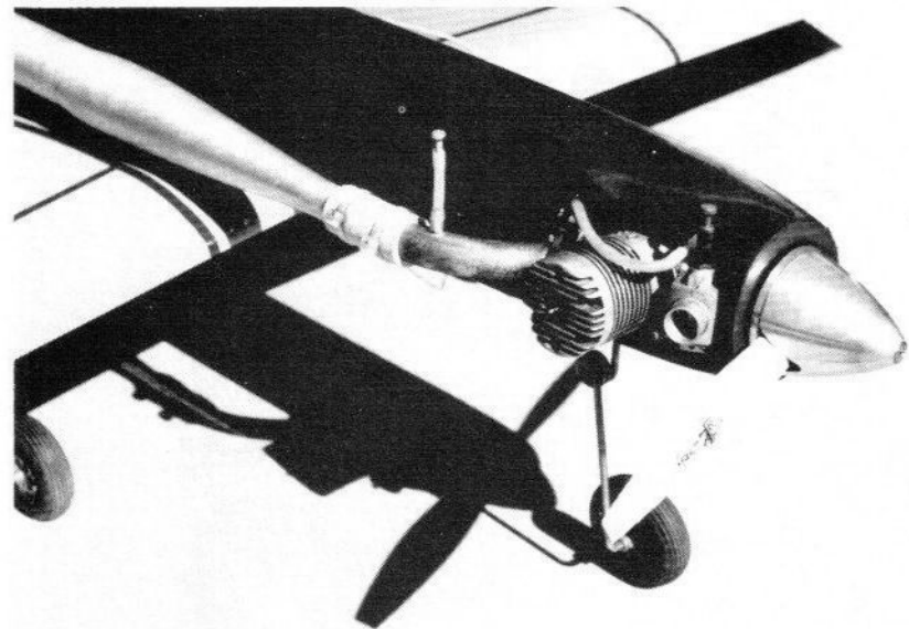
O.S. 60 installation shown with Mac header and pipe.
