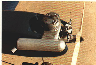
K&B Sportster installation—a good choice for the Senior. Wide speed range of this model will suit any pilot.
