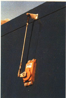
Eflon servo position when using an electronic mixer in transmitter or receiver. Model is very directional.
