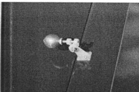
Method of elevon balance, 1/2 ounce sinker, link from elevon and cut down large control horn.
