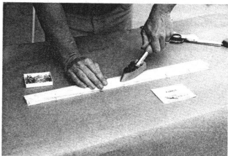
Iron X-hinge down on elevon (both sides).
