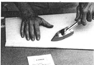
Pin elevon in place on wing and iron X-hinge down on both sides.
