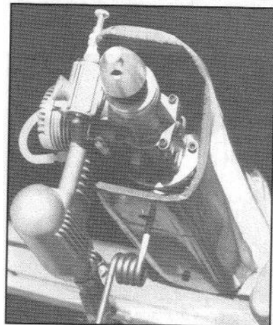
LEFT: Detail of K&B .40 mounted with Evans EZ Mount. RIGHT: Canopy detail.
